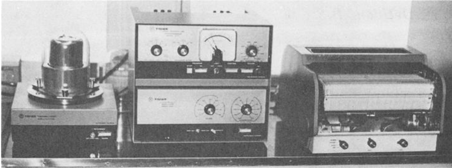
FIG. 1—Quantitative DTA system with recorder.
